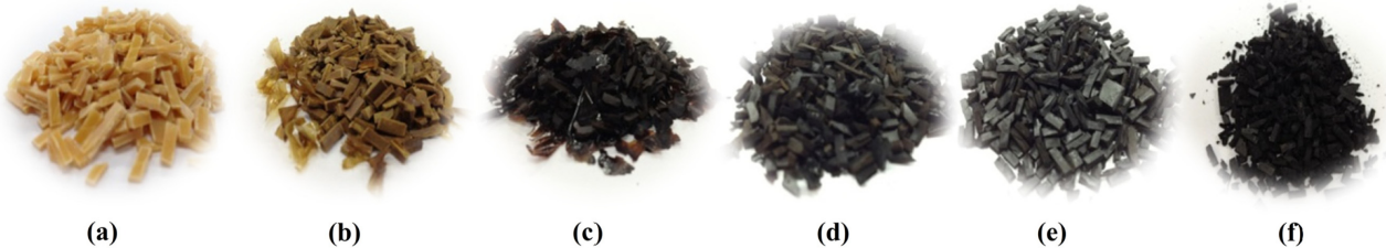
Fig. 2. Photographs of phenol resin after treated with various supercritical solvents; (a) raw phenol resin (b) methanol, 280 °C, 147 bar (c) methanol, 380 °C, 223 bar (d) ethanol, 380 °C, 177 bar (e) acetone, 380 °C, 125 bar (f) water, 380 °C, 219 bar.
