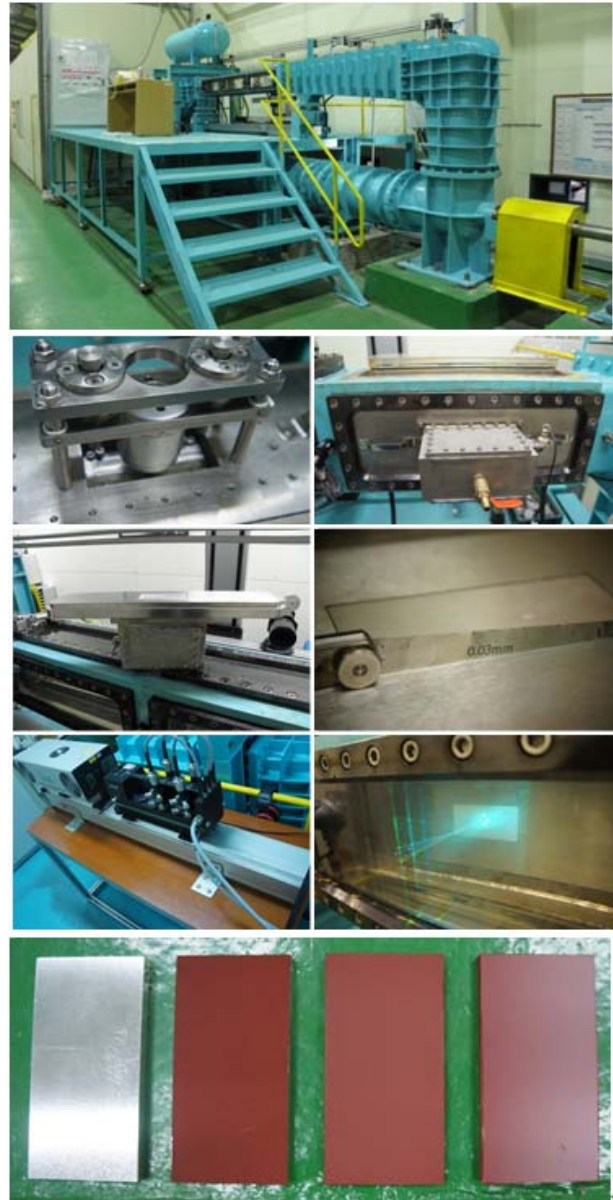
Fig. 2 Photos of the high-speed water tunnel, flush-mounted balance and the samples of FDR-SPC and FDR-AF coatings
