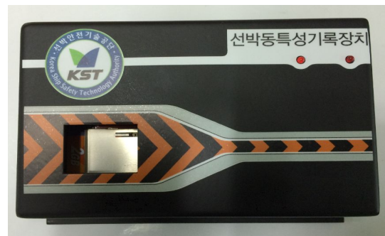
Fig. 4. Ship's data recorder of dynamic characteristics.
