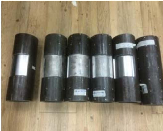
Fig. 8. The specimens for test of wall-thinning effect on eigenfrequency change of straight pipes.
