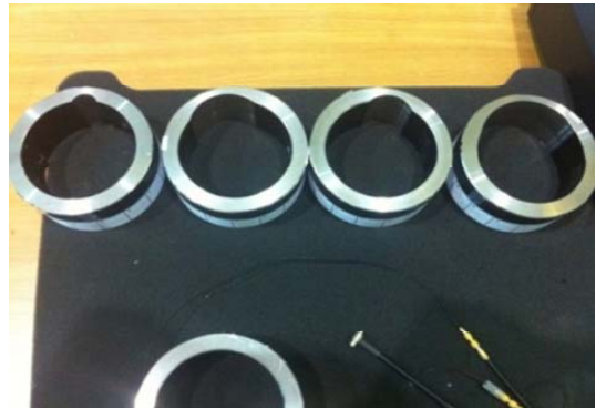
Fig. 4. Test specimens of wall-thinned pipes with short axial length
