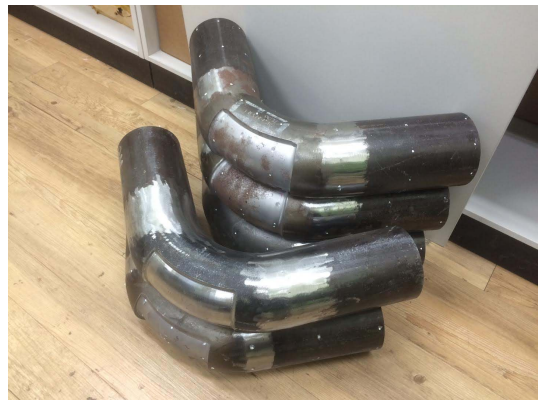
Fig. 11. Test specimens of wall-thinned curved pipes.
