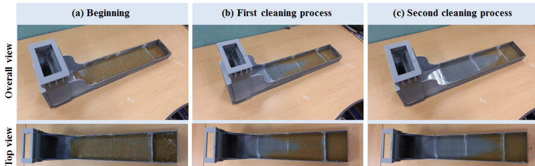
Fig. 3 State of the sediment on the bottom of the retention basin depending on the cleaning process step (the radius of bucket: 0.5 m and the bottom slope: 5.0 %)
