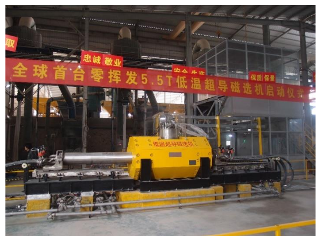
Fig. 7. The first CGC-5.5/300 HGMS system at Quanzhou City, Fujian Prov.
