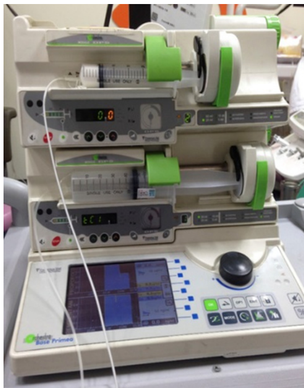
Fig. 2. The target controlled infusion pumps are used to administer propofol and remifentanyl.
