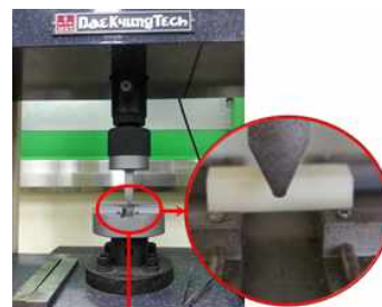
Fig. 6 3-point bending test
