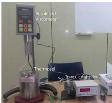
Fig. 4 Binder viscosity measurement system
