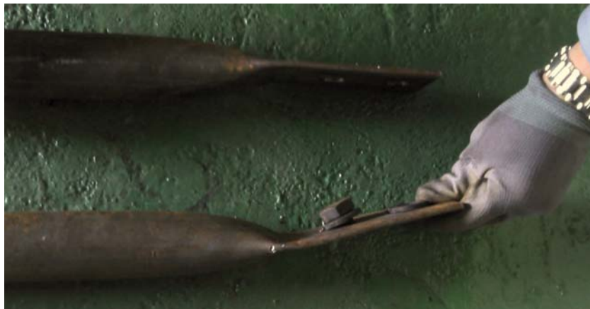
Fig. 6. Apparent test for straightness at connecting zone.
