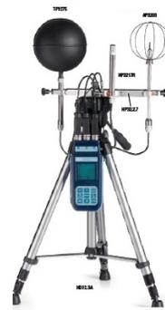
〈Fig. 2〉 Thermal comfort measurement (Delta ohm)
