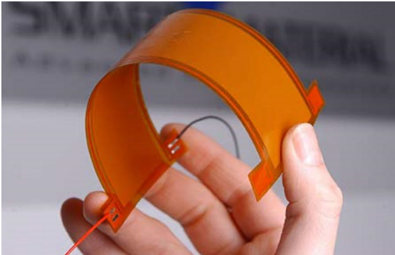
Fig. 4. Example of MFC piezoelectric actuator [15]
