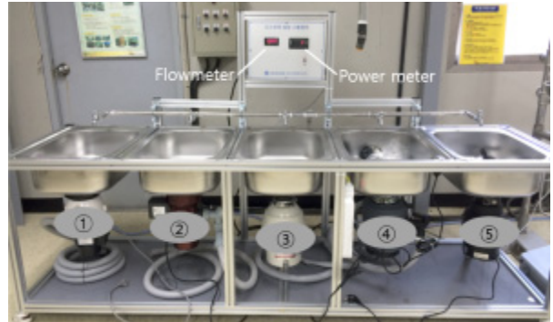
Fig. 2 Experimental apparatus of a food waste disposer
