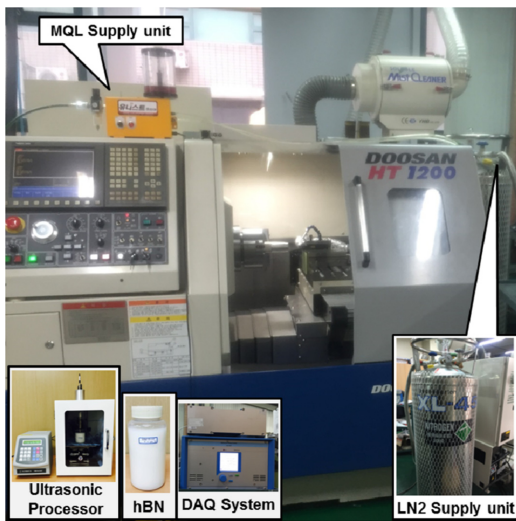
Fig. 1 Entire experimental system with cryogenic cooling (LN2) and nanofluid (hBN) MQL supply units
