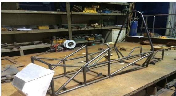
Fig. 4 A new frame of the 2016 model
