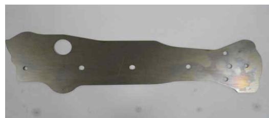
Fig. 16 Blank size of seat track
