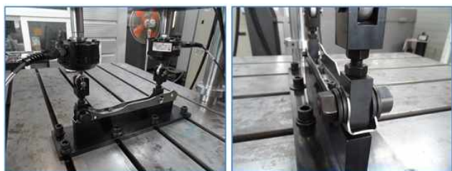
Fig. 19 Durability test of seat track
