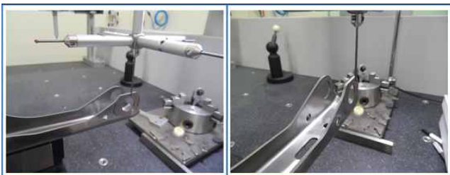
Fig. 18 3D dimension measurement of seat track
