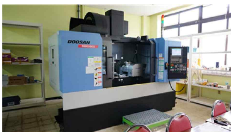
Fig. 3 Machining center with FANUC controller
