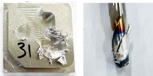
Fig. 16 Failed machining (trochoidal-level 4, depth 12 mm)
