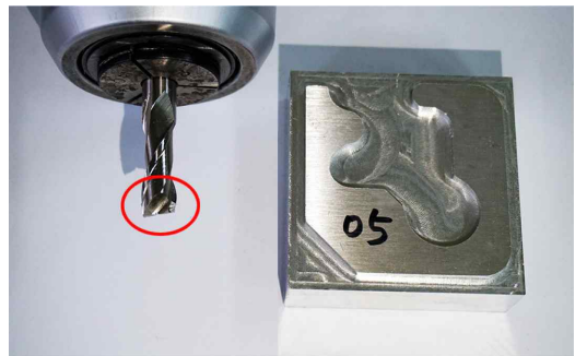
Fig. 9 Tool broken (contouring-level 5, depth 3 mm)
