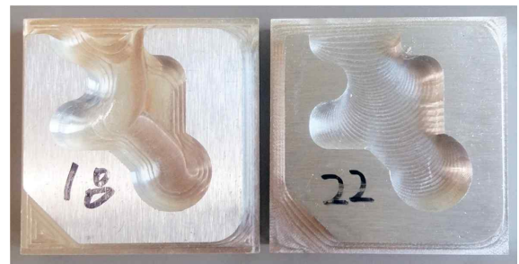
Fig. 13 Differences between contouring and trochoidal
