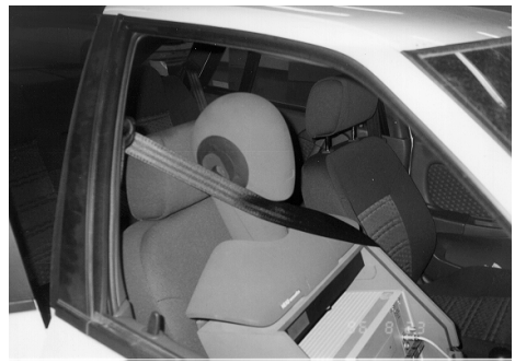
Fig. 1 Dummy Head installed at assistant driver seat
