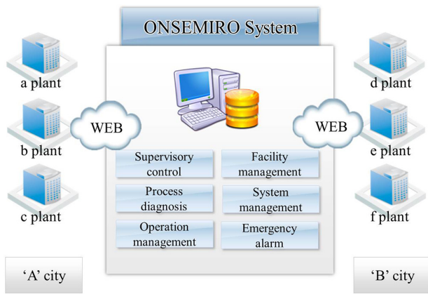
Fig 1. Schematics of ONSEMIRO system
