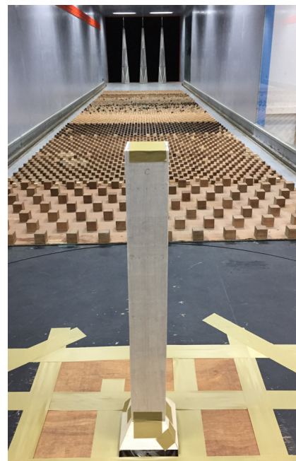
<Fig. 1> Pressure taps (Taps are not installed on Surface B and D) and setting of model
