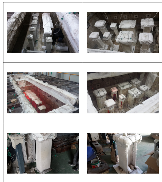
<Fig. 3> Specimens after fire test
