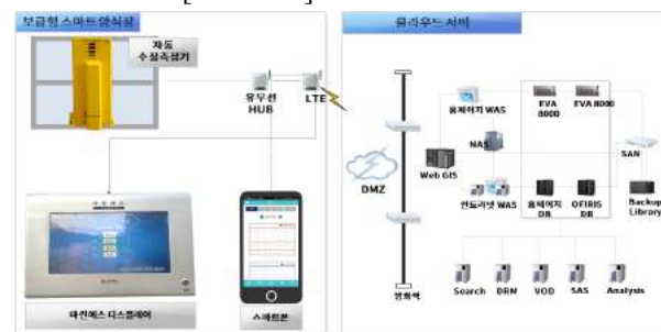
picture 3 System diagram of IoT-based non-cleaning water quality measuring equipment
