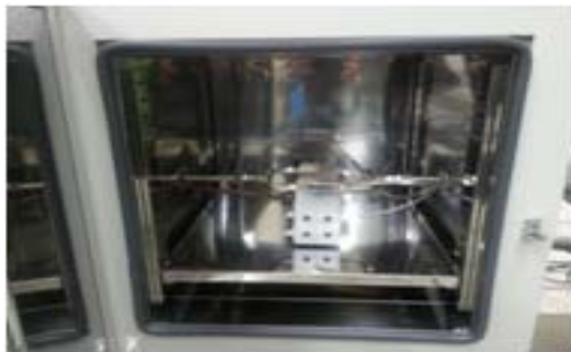
Fig. 5. NG Blower operation in chamber.
