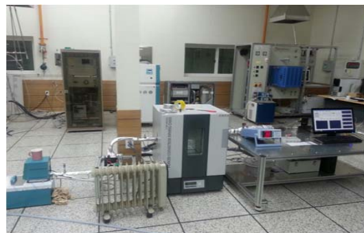
Fig. 4. NG Blower performance evaluation apparatus.
