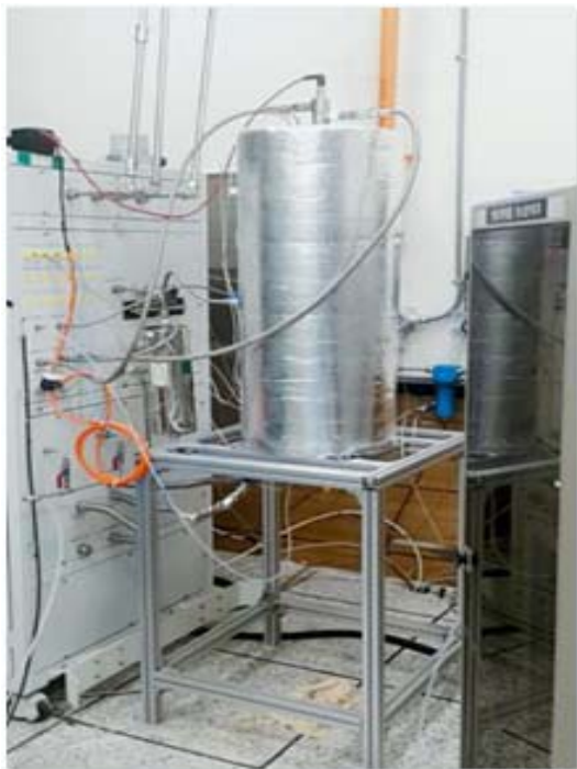
Fig. 10. Picture of improved fuel processor.
