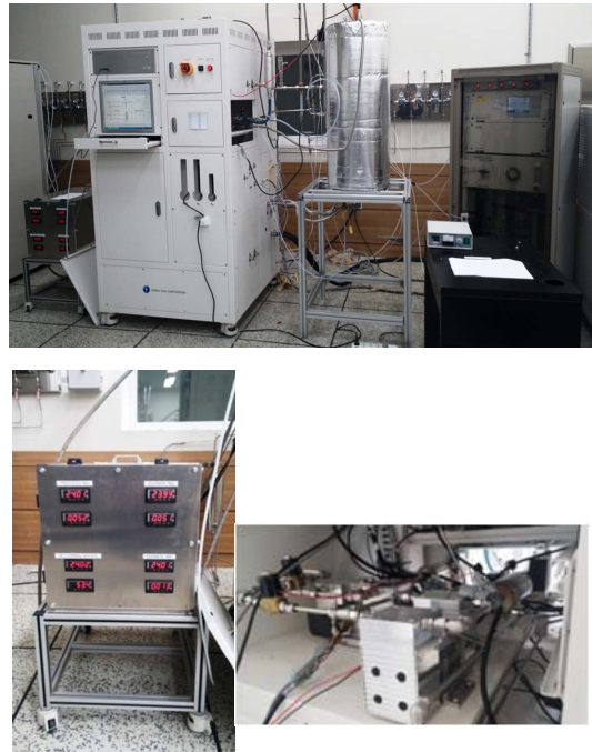
Fig. 13. Fuel Processor module performance evaluation apparatus.
