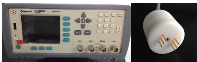
Figure 1. Photograph showing the impedance machine (left) and the probe (right) used in this work.
