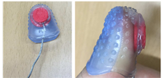
Fig. 3 Force sensing module (a) feature of force sensing module (b) wearing force sensing module
