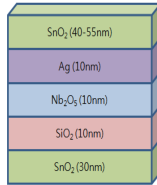
Fig. 1. A schematic diagram illustrating the structure of \text{SnO}_2/\text{Ag}/\text{Nb}_2\text{O}_5/\text{SiO}_2/\text{SnO}_2 multi layer film.
