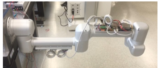
Fig. 1. 6-DOF manipulator in press forming process
