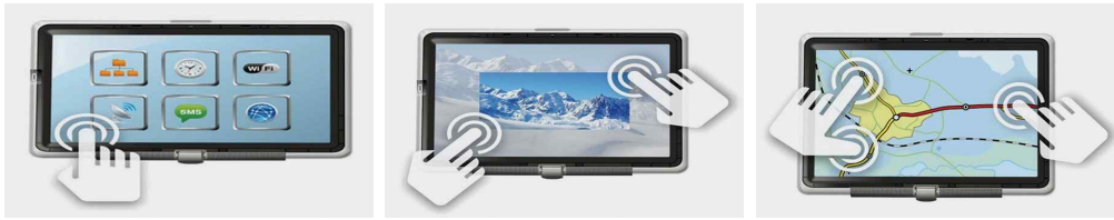
Fig. 1. The forms of touch interface: single-touch, multi-touch gesture, multi-touch all-point.
