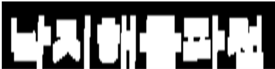
Fig. 7. Vertical blur-applied binary image
