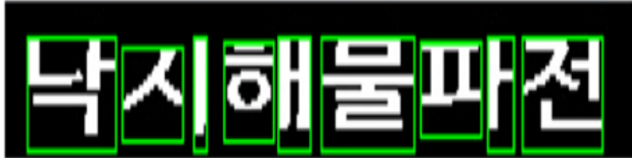
Fig. 8. Labeling algorithm application to Fig. 4 image to group neighboring pixels
