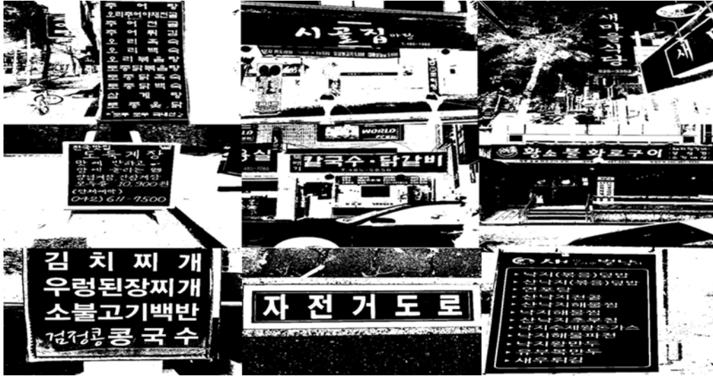
Fig. 17. Test result of binarization algorithm for text area detection in outdoor environments
