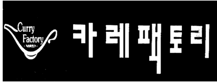
Fig. 5. Niblack binarization algorithm-applied image after lighting removal
