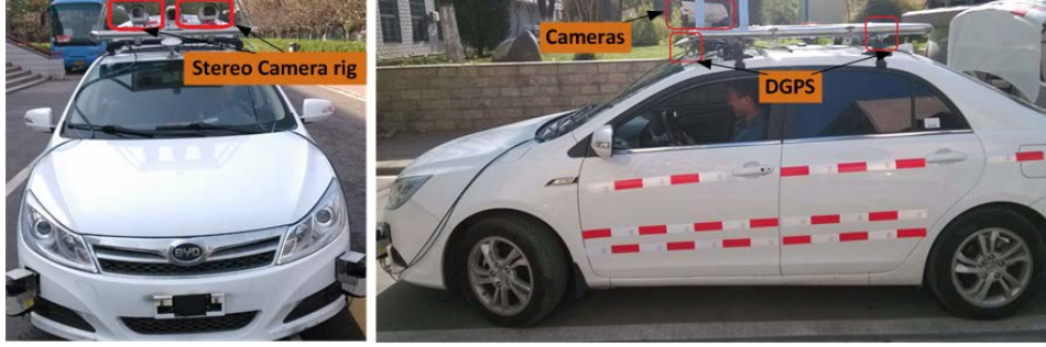
Fig. 1. Experimental platform with vehicular stereo camera rig and DGPS.
