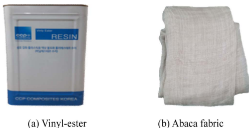
Fig. 1. Matrix and reinforcement
