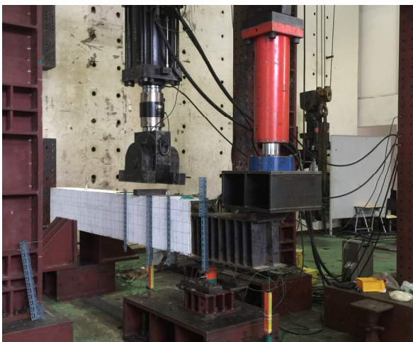
Fig. 5 Test set-up (one-way shear specimen)
