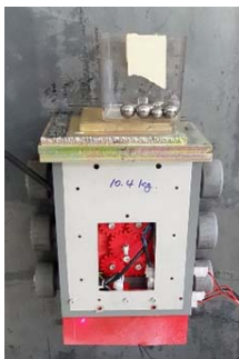
Figure 10: An example scene of measuring the slip of a wall-climbing robot against adding load
