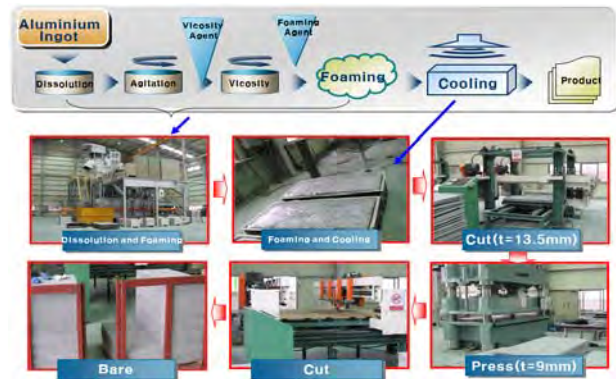
Figure 1: Foamed Aluminum Process
