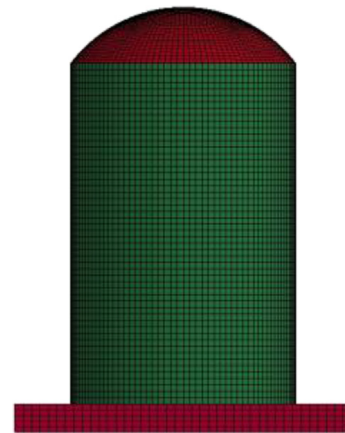
Fig. 10. Numerical model of containment vessel specimen.
