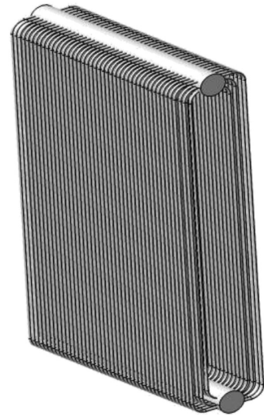
Fig. 4. Schematic diagram of a passive containment cooling system (PCCS) heat exchanger (PCCX).
