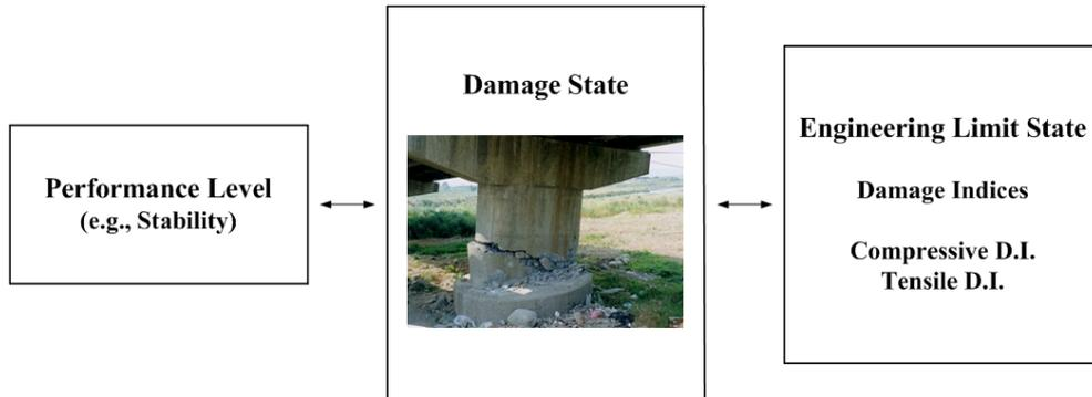
Fig. 13. Links between performance level, damage state and engineering limit state [13]
