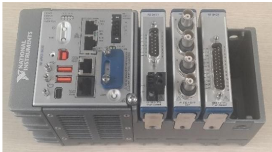
Fig. 8 CompactRIO-9033 and I/O module of National instrument
