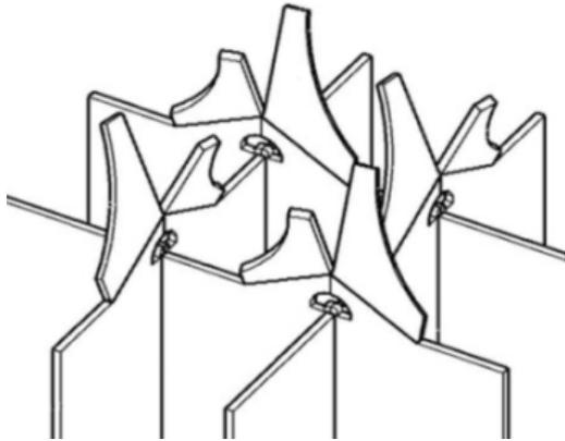
Fig. 2 Schematic diagram of twist-vane spacer grid<sup>(11)</sup>
