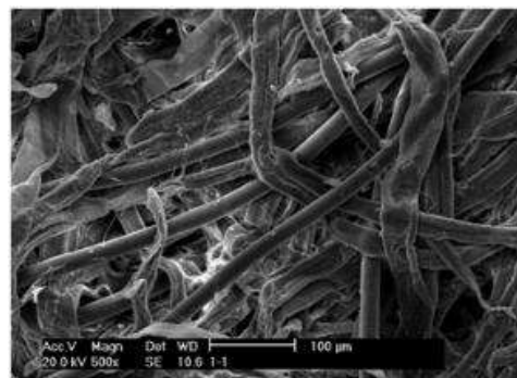
Fig. 3 SEM photo of the paper used in the present indirect evaporative cooler
