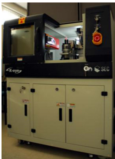
Fig. 1. X-ray CT scanner at KICT
