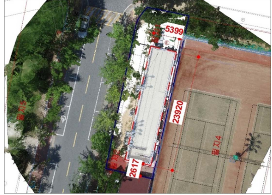
Fig. 6 Image Matching & Geometric Correction Using GCPs
