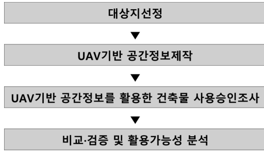
Fig. 3 Process of Experiment for Automated Inspection for Building Occupancy Authorization
