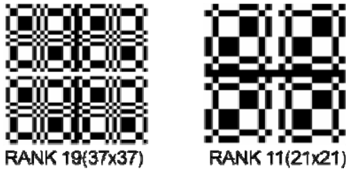
Fig. 1. Simulated collimator pattern (MURA).
