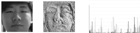
Fig. 2. LBP Processing and Color Information for Face Recognition
