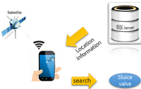
Fig. 3 Sluice valve location matching process
