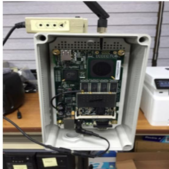
Fig. 5 AP for developed drone network
