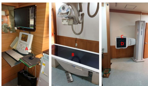
[Fig. 2] Sample collection from 4 places in general x-ray room in the radiology department, sample collection from exposure controller (A), patient table (B), stand bucky-chin support (C) and stand bucky-grid (D) of general radiographic system.
