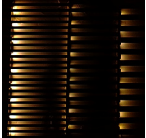
Fig. 8. F1=1kHz, F2= 1.5kHz, F3=2kHz, d=5cm, FOV=90 on rolling shutter image sensor
