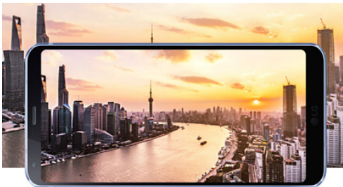
Fig. 1. Trend of screen-to-body ratio of mobile phone (Upper), and full screen image of the LG G6 which exhibits screen-to-body ratio of 80.70% (Lower)[2,3].
