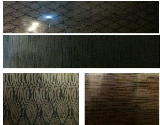
Fig. 3. Implementation of UV mold pattern designs of optical illusion for real emotional furniture, which was performed with roll-to-roll process. The upper images are 200 cm width and 50 cm height, The lower images are detailed patterns of upper images.
