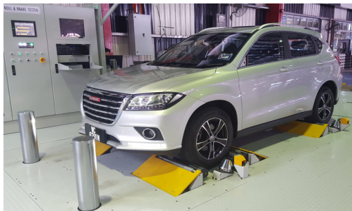
Fig. 8 Vehicle on Roll and Brake tester
